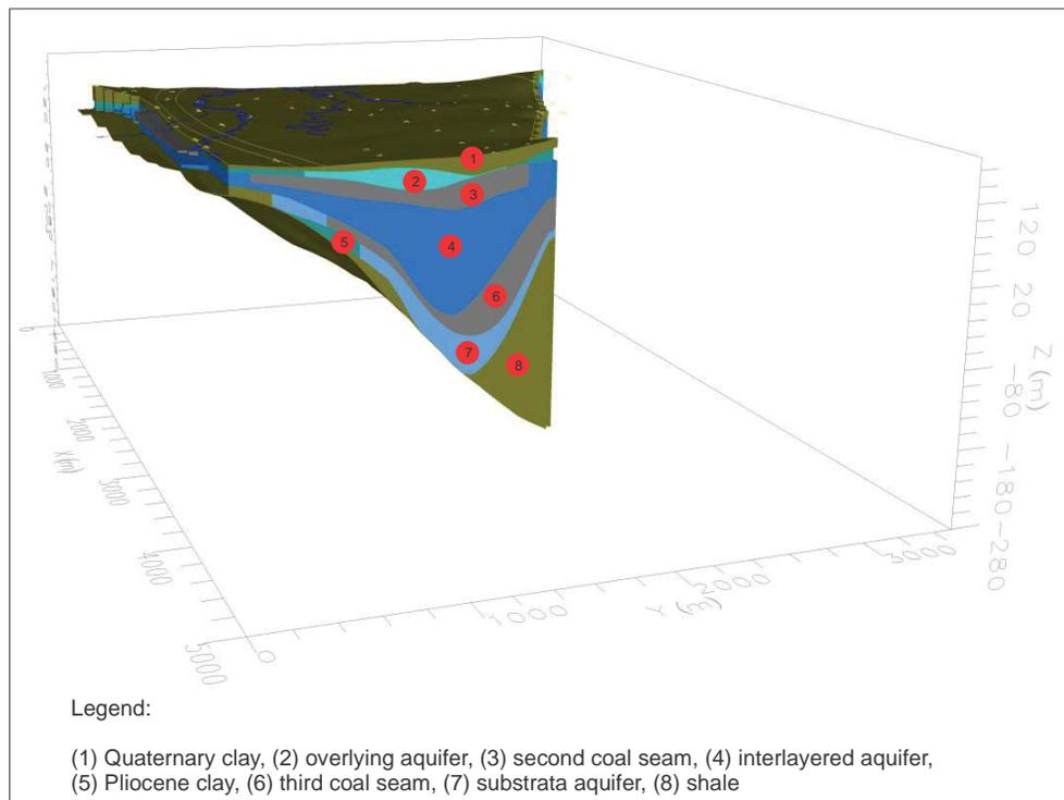
**Fig. 8.** Hydrogeological profile of strike west-east
