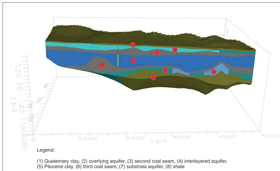
Fig. 7. Hydrogeological profile of strike south-north
