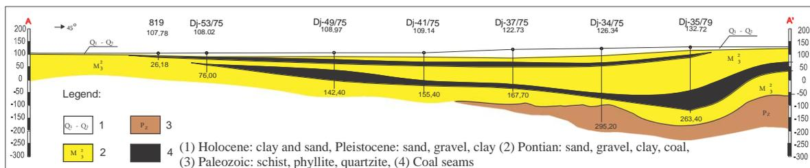
Fig. 3. Geological profile A-A'
